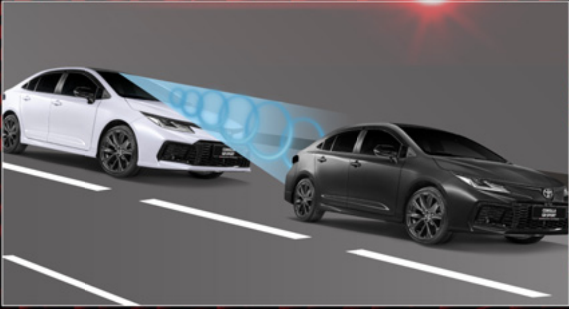
DYNAMIC RADAR CRUISE CONTROL (DRCC) FOR ALL SPEEDS* Maintains a safe distance with preceding vehicle and brakes automatically when the car ahead stops.
