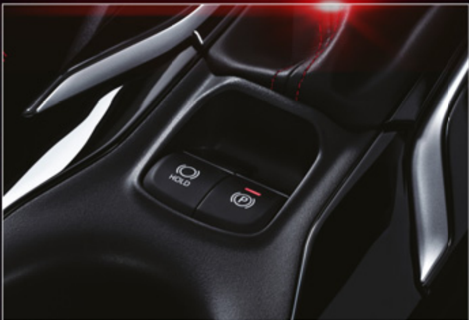
ELECTRIC PARKING BRAKE (EPB) WITH AUTOMATIC BRAKE HOLD Keeps the vehicle stationary on flat roads with a simple button. Automatic release during acceleration.
